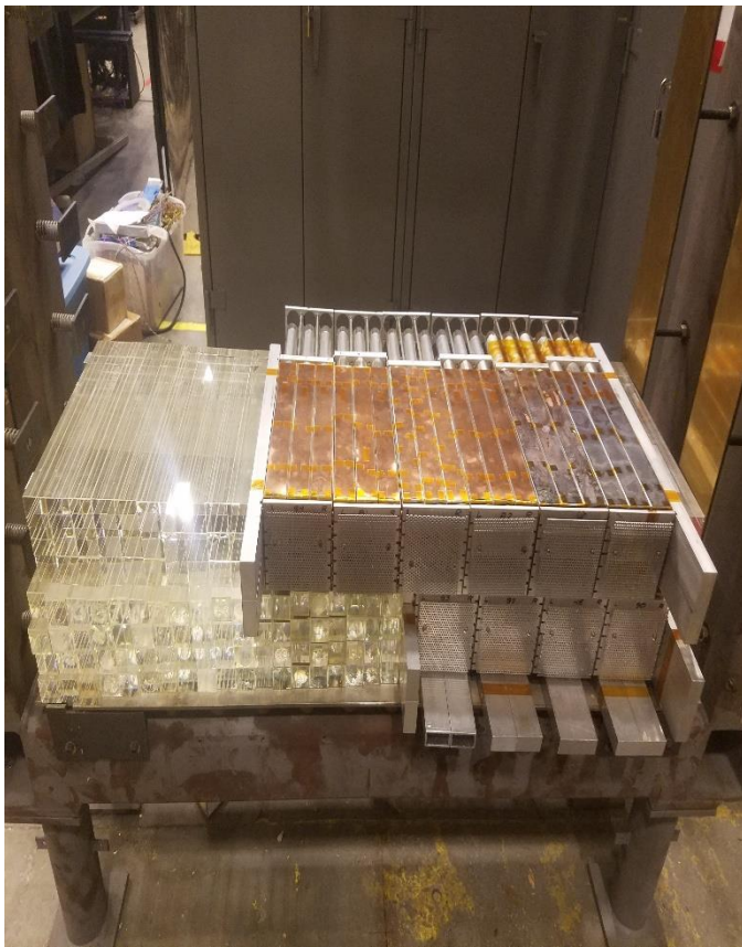
Ecal Frame with 2 layer Super Module front
