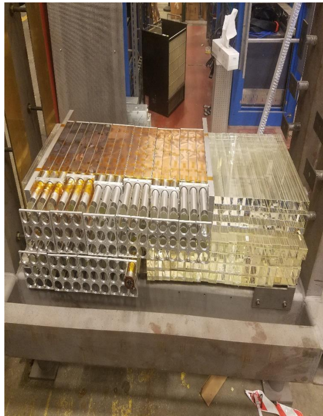
Ecal Frame with 2 layer Super Module back
