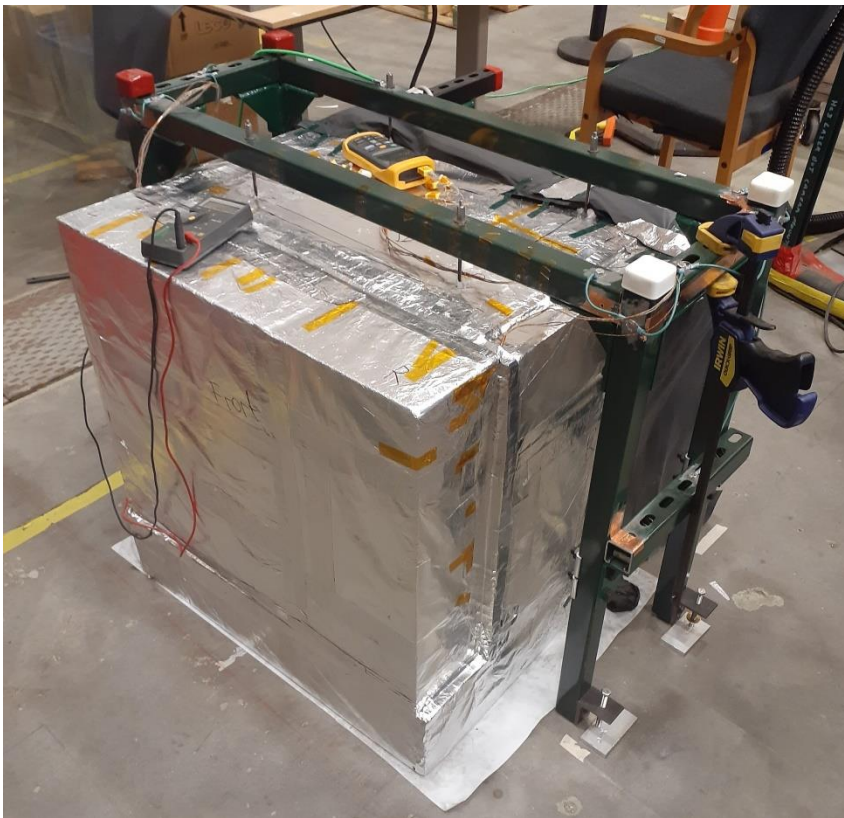
Prototype covered with foam-glass Front view
